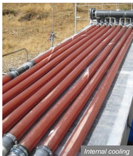
Figure 10 Pilot scale panel photobioreactor (4x25 L) and pilot scale tubular photobioreactor (65 L) in Aachen, Germany and Ankara, Turkey, respectively.
